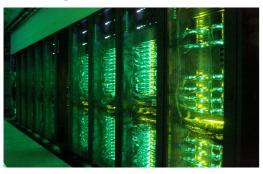
For scalable parallel performance, the system is equipped with high bandwidth, low latency FDR/EDR InfiniBand interconnects.
